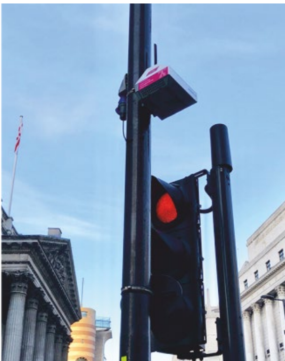
Graphic 2.2 Example of a real-time particulate monitor
